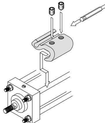
• The above figure shows the mounting example of D-A9□(V)/M9□(V)/M9□W(V)/M9□A(V)L.
