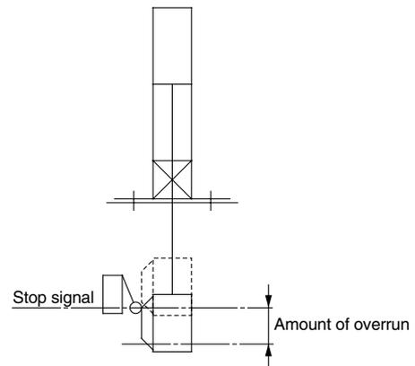
3. In order to further improve stopping accuracy, the time from the stop signal to the operation of the lock should be shortened as much as possible.
