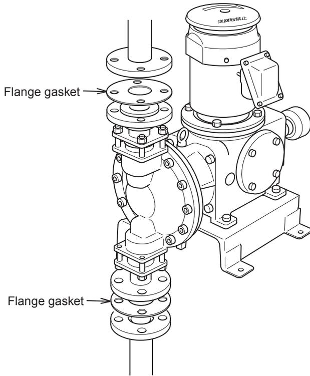
6. Connect the suction and the discharge lines to the inlet and the outlet over the gaskets. Tighten the flange bolts to the same torque in diagonal order.
