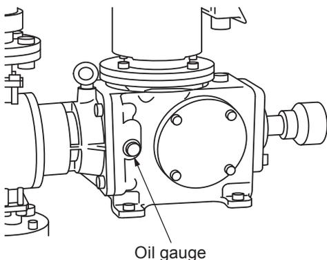
1. Check for transit damage, loose bolts and an oil leak.
