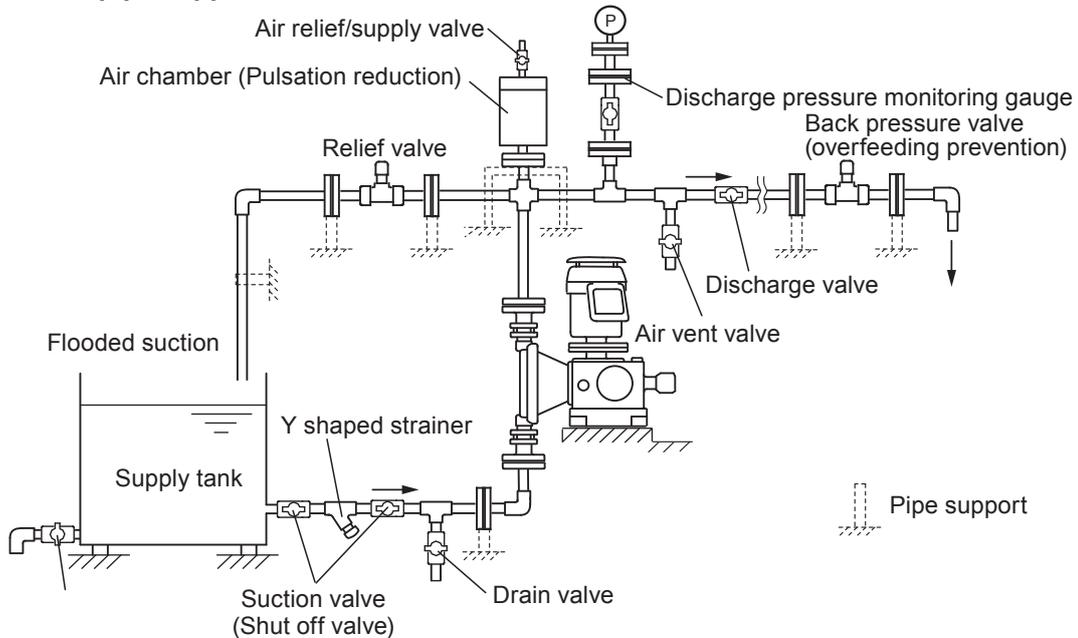
NOTE: Design an efficient layout to meet NPSHr, especially when planning to deliver slurry.
