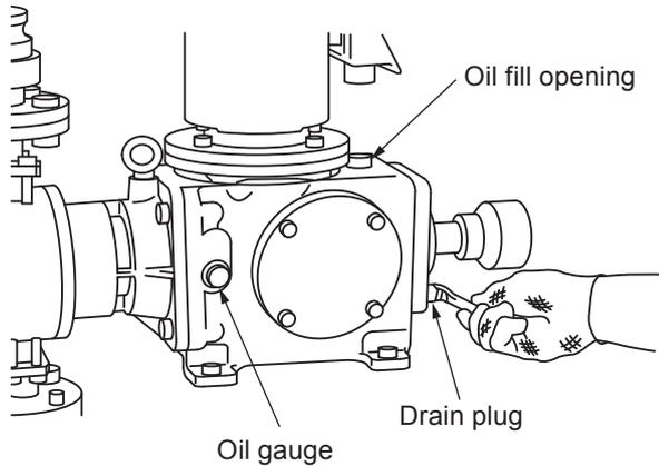
1. Loosen the drain plug and release old oil.
